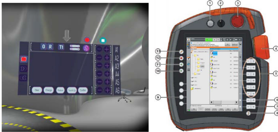
Figure 2: The virtual input panel closely mirrors the design and layout of the Kuka SmartPAD.
