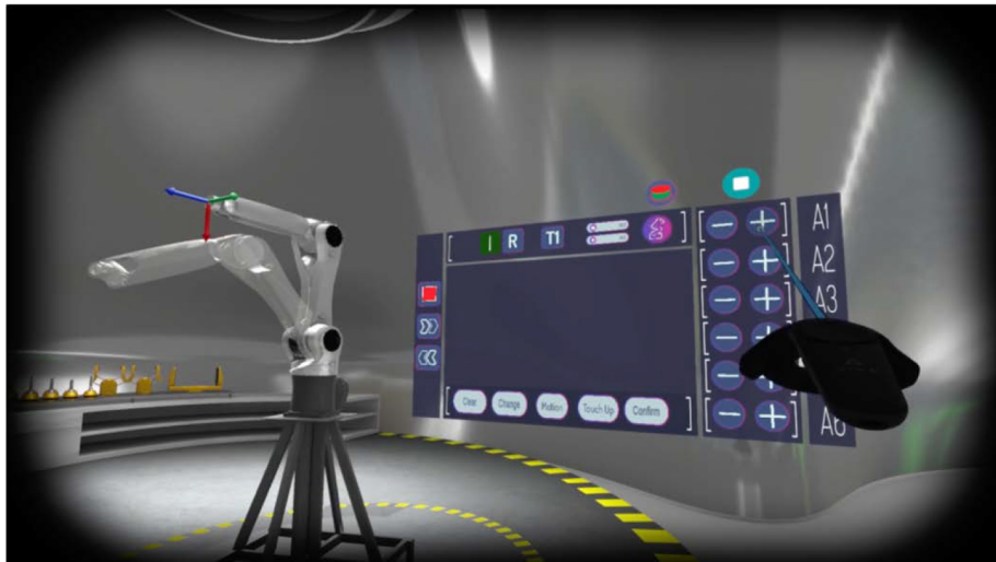
Figure 3: Students are challenged to match the position and orientation of a “ghosted” robotic arm using both Axis-specific and World-specific motion systems.
