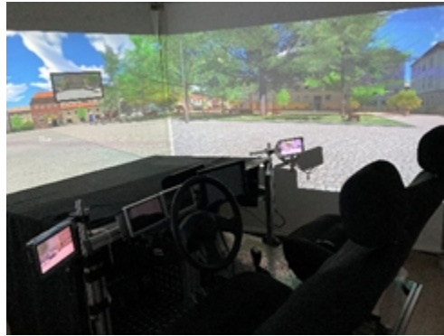
Figure 1: Stationary driving simulator of the TU Braunschweig with running simulation.
