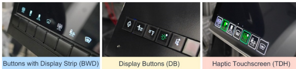
Figure 3: The three potential digital input modalities as interactive prototypes with a rudimentary adaptive user interface.
