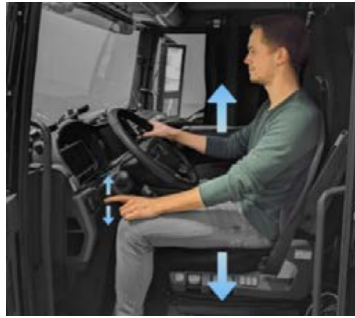
Figure 1: Moving seat fitted to a truck cockpit which introduces vertical movement into the driver's body and limbs, therefore making it harder to reach for control elements.
