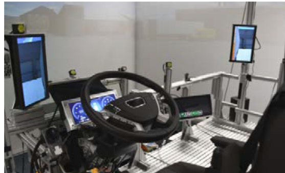
Figure 4: Static truck driving simulator running with eye tracking cameras and integrated TDH prototype.
