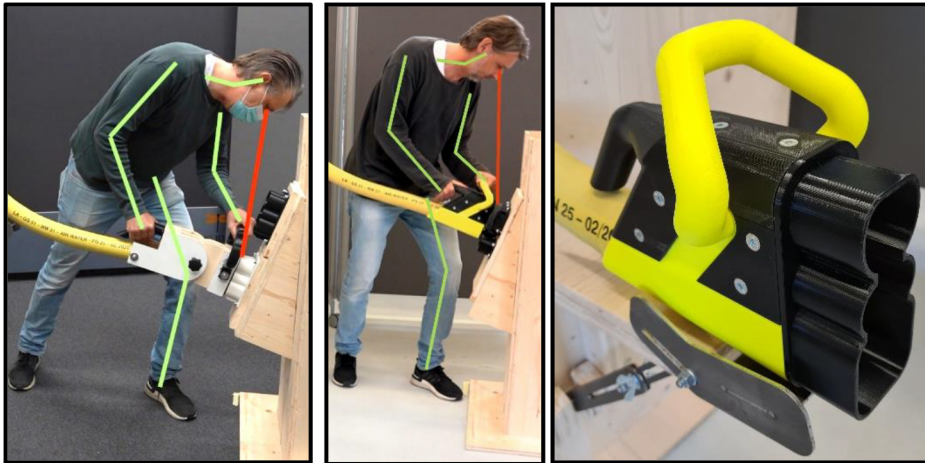
Figure 2: Left: 98% man using ergonomic model of first test series, centre: 98% man using improved model within comparative study, right: Improved one-plug solution.
