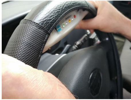
Figure 1: Steering wheel cover deployed. The electrodes have an identical look and feel to that of a regular cover; a visual analog scale (VAS) placed at the center of the steering wheel, following a color-coded simplified version of the karolinska drowsiness scale (KDS).
