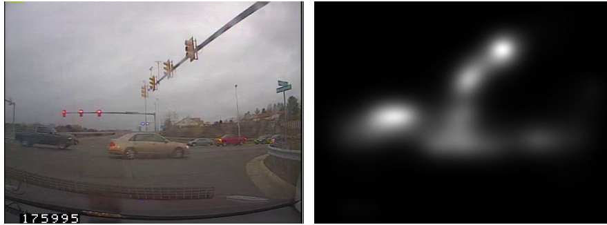
Figure 1: Object saliency for roadway scene. This shows that the saliency of any scene is generally targeted to the objects present in the scene. Higher intensity refers to higher value of saliency (Cornia et al, 2018).
