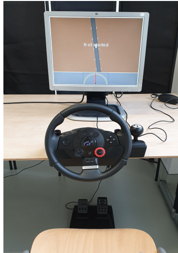
Figure 2: The experimental setup as seen from the view of one participant. The participant sees a top-down view of the vehicle they can control with the gas and brake pedal. The steering wheel provides vibration feedback if the participant deviates from the designated velocity. Visual velocity feedback is provided through the speed dial in the lower part of the screen.
