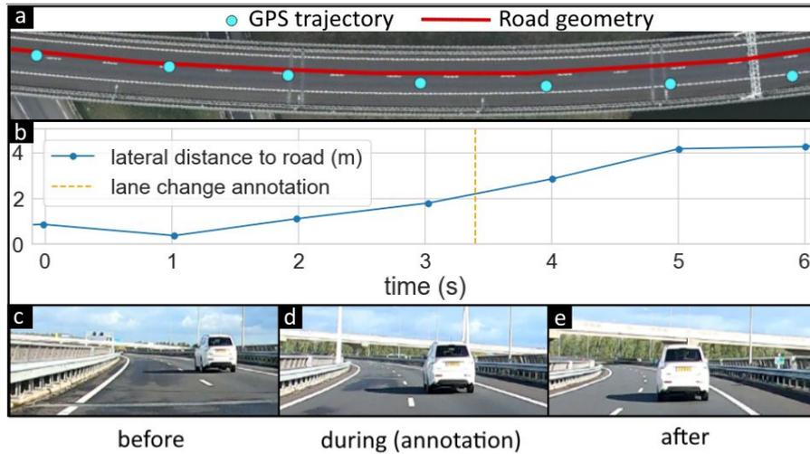
**Figure 3:** a: Map view of road section with a lane change. b: Lateral distance of the GPS points relative to the road during the lane change (in meters). c, d, e: Video segments of the lane change from the perspective of the ego vehicle, where panel (d) shows the moment the lane change was manually annotated (the camera view is visually centered with the lane boundary).
