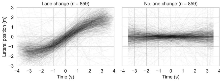
**Figure 4:** Left: Lateral position relative to the segment's mean for all lane changes and all four devices ( $n = 215$  lane changes  $\times$  4 devices  $- 1$  missing segment = 859). The lane change took place at Time = 0 s. Right: Lateral position relative to the segment's mean for segments in which no lane change took place.
