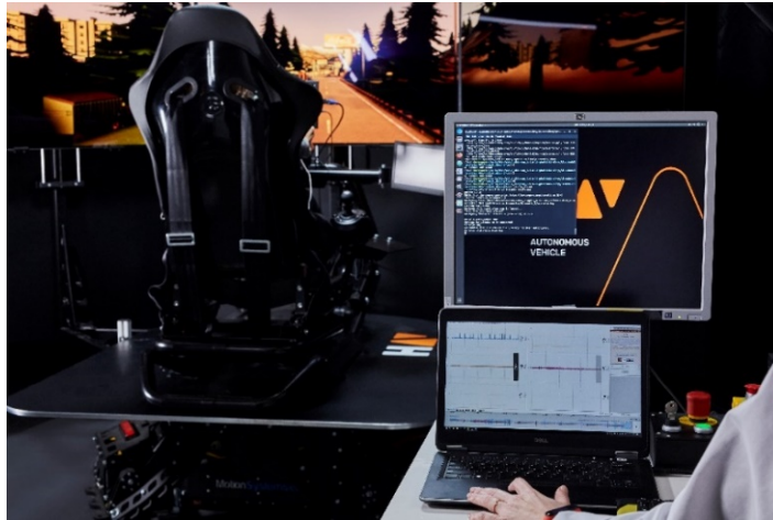
Figure 3: Technician launching a scenario and measuring physiological signals.
