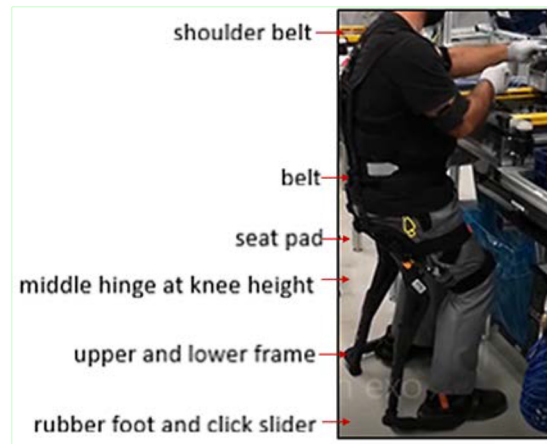
Figure 1: Lower body exoskeleton – Chairless chair 2.0 (CC 2.0). Exoskeleton was used in Experiment 2 (EXO): minimizing the physical load by ergonomic sit-stand pattern.
