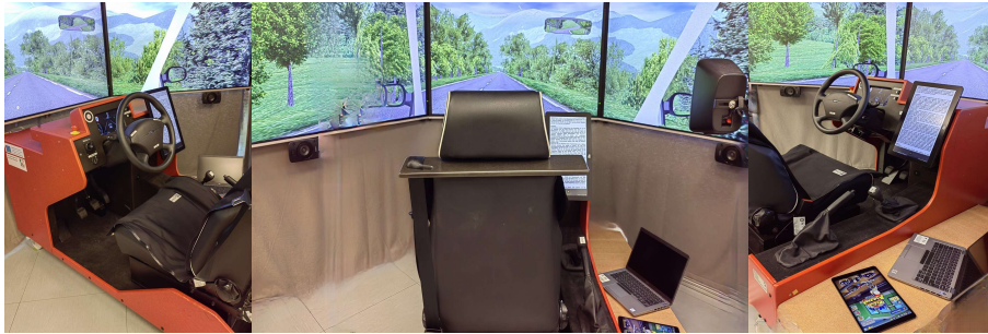
Figure 1: The experimental setup for acquisition of driver activity data.
