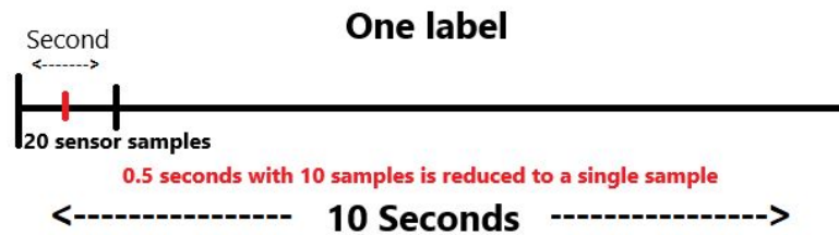
Figure 4: The amount of data is compressed to 2 Hz from the original dataset with 20 Hz.
