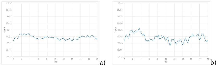
**Figure 5:** Evolution of the temperatures of the cold thermoreceptor ( $T_c$ ), for an air velocity random in the occupant's neck area. Figure a) is associated to the Case A and figure b) is associated with the Case B.
