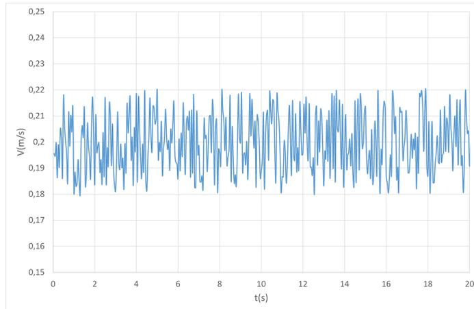
**Figure 2:** Air velocity random signal used in the human thermal response numerical simulation in the Case A.
