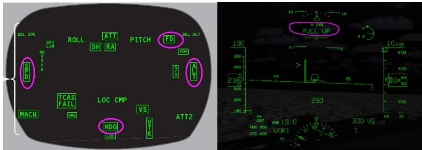
Figure 2: Failure flags of HUD warning.
