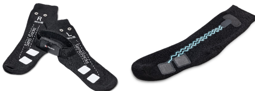
Figure 6: Sock garment with electronics module on the outer side (left) and inner side (right).
