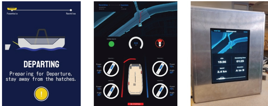
Figure 3: (a) Design A simple information display; (b) Design B technical information; (c) prototype of the passenger information screen.
