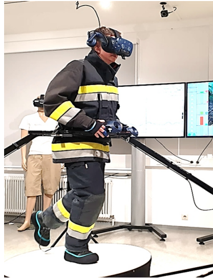
Figure 1: First responder in the treadmill with biosensor evaluation kit for the VR-based study of SA in critical situations (credit: L. Paletta, JOANNEUM RESEARCH DIGITAL).
