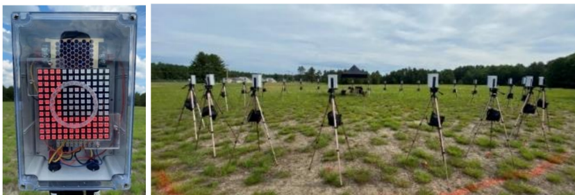
Figure 2: Example light box target with LED screen displaying a shape that represents an enemy threat (left), placed on stands in a 360-degree circle (right) (courtesy of Brown et al., 2022).
