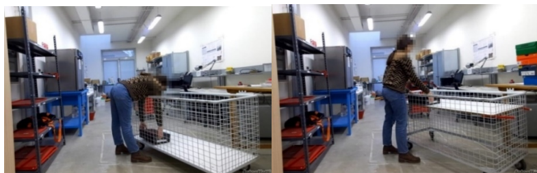
Figure 2: Lifting action with fixed mesh truck (left) and lifting action with height-adjustable mesh truck (right).
