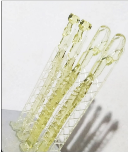
Figure 12: Resin printed prototype in creality Ld 002h.
