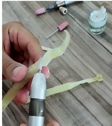
Figure 18: (Right) grinding the prototype in resin.
