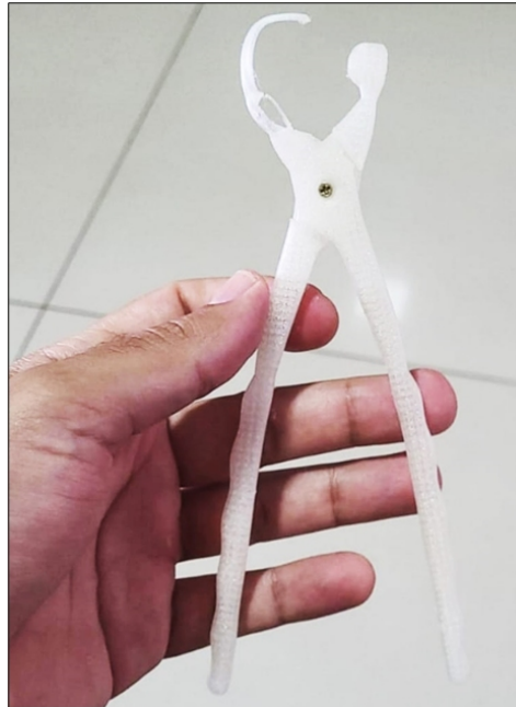
Figure 15: Handle of the prototype printed in PLA.
