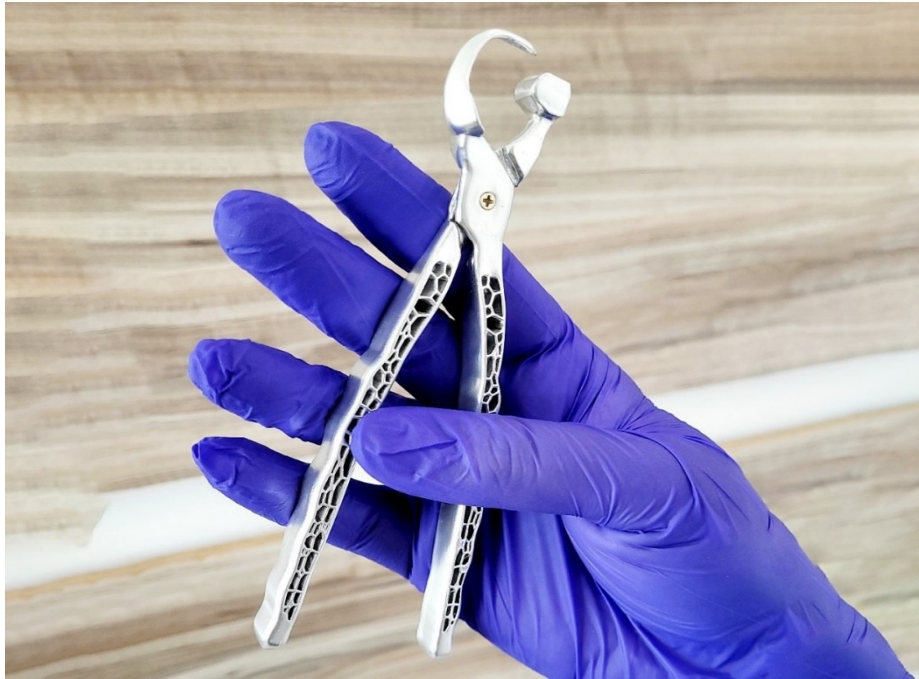
Figure 13: Final prototype printed in resin.
