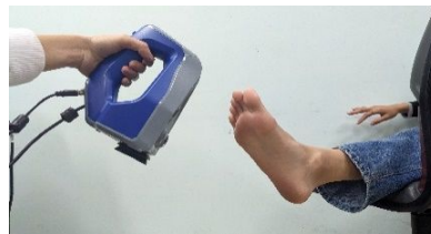
Figure 6: Scanning the subject's foot with the artec space spider 3D scanner.
