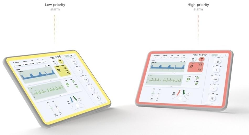
**Figure 7:** Digital interface of the new ventilator, which communicates the detected problem to the user through visual and audio feedback.
