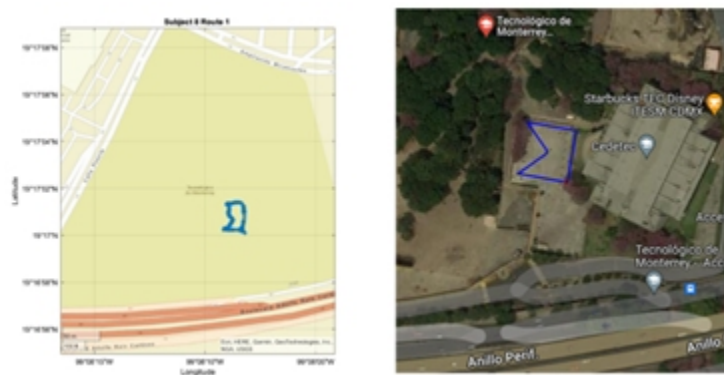
Figure 7: GPS module mapping of Subject 8 trajectory 1 in comparison to the ideal pattern traced from the trajectory designs.
