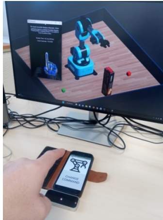
Figure 4: Leap Motion used to interact with a virtual robot without touching the smartphone.
