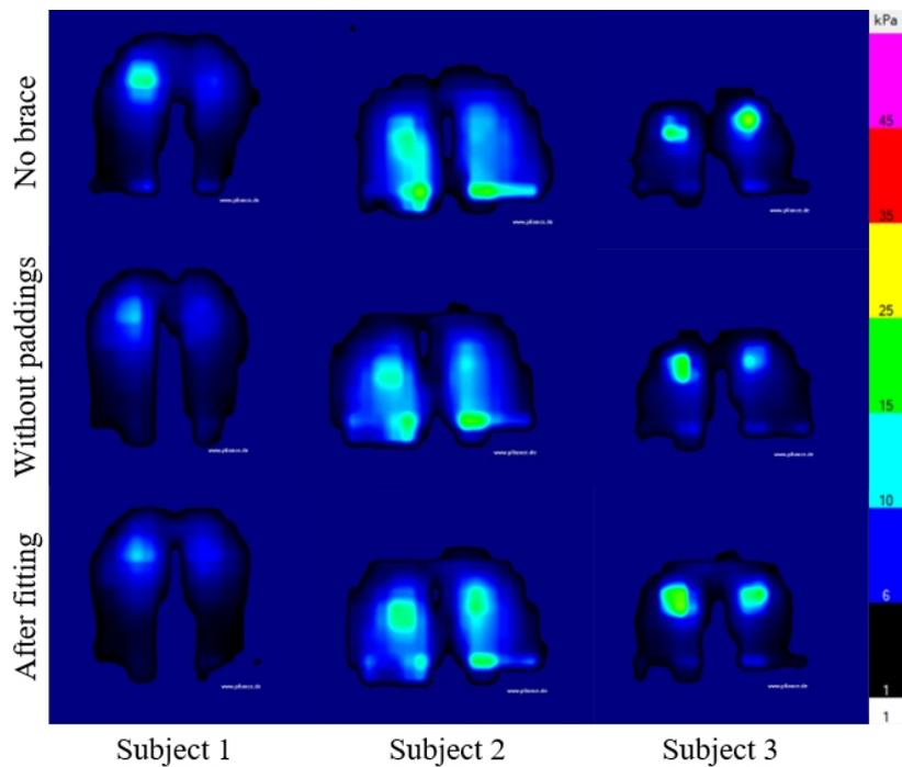
**Figure 5:** Sitting pressure distribution for each subject: without the brace, without paddings, and after the pressure fitting.
