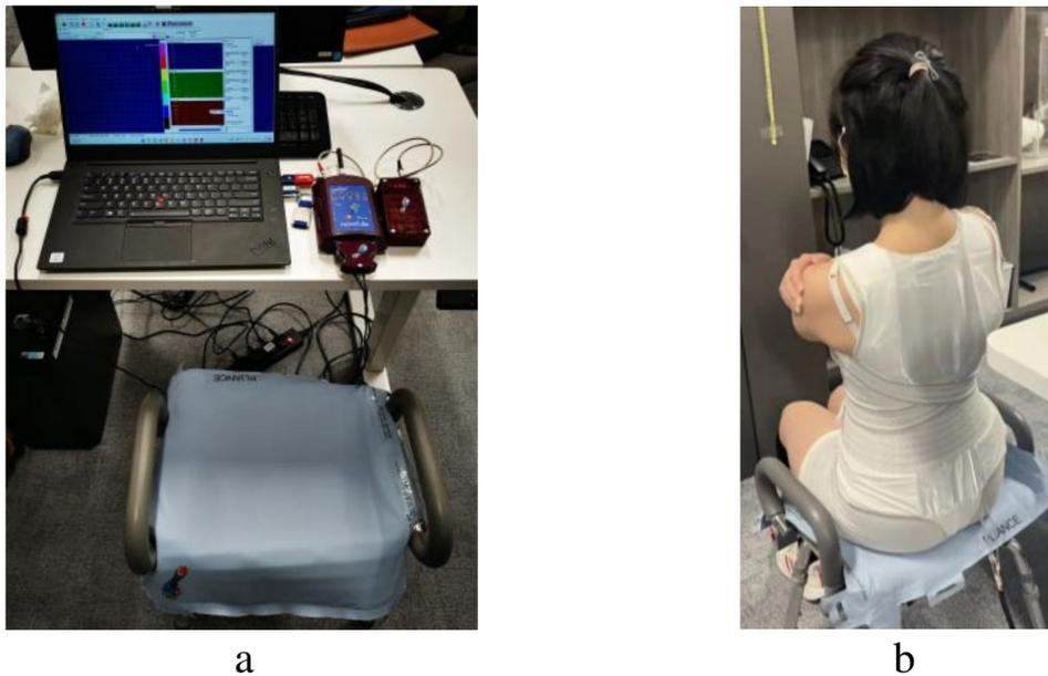
**Figure 3:** Sitting balance measurement: a. pliance system and b. sitting measurement.
