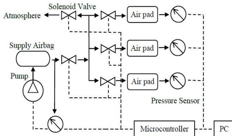
**Figure 2:** Control diagram of the pneumatic padding system.
