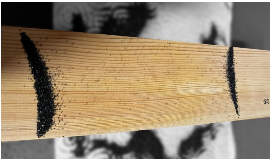
Figure 1: Chladni test performed on a maple table. (Photo: Ermanno Aparo, 2023).
