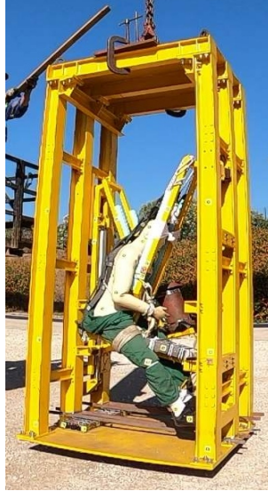
Figure 4: Free fall tests on a full-scale shelter section with a crash test dummy.
