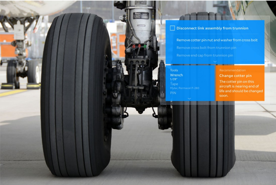
Figure 3: Screenshot of CHEWBACCA’s AR interface for aircraft maintenance.
