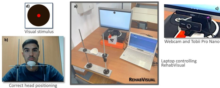
**Figure 1:** RehabVisual experimental setup, displayed in the centre, a). The lower-left frame, b), contains an example of use of the chin-immobilizer, whereas the upper-right one, c), zooms in on the webcam and Tobii eye tracker. On the upper-left corner, d), is displayed the visual stimulus employed throughout the experiments.
