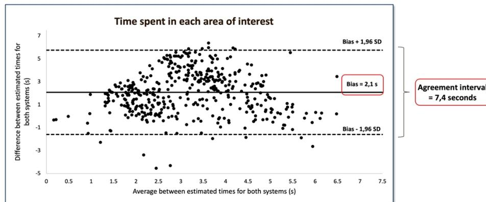
**Figure 4:** Bland-Altman plot for the overall agreement between time spent in all the pre-defined areas of interest, for both the RehabVisual and the Tobii Pro Nano eye trackers. The bias between both models and the 1.96 standard deviations are also marked.
