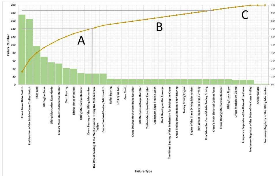
Figure 2: Pareto diagram of failures and stoppages for transport machinery.
