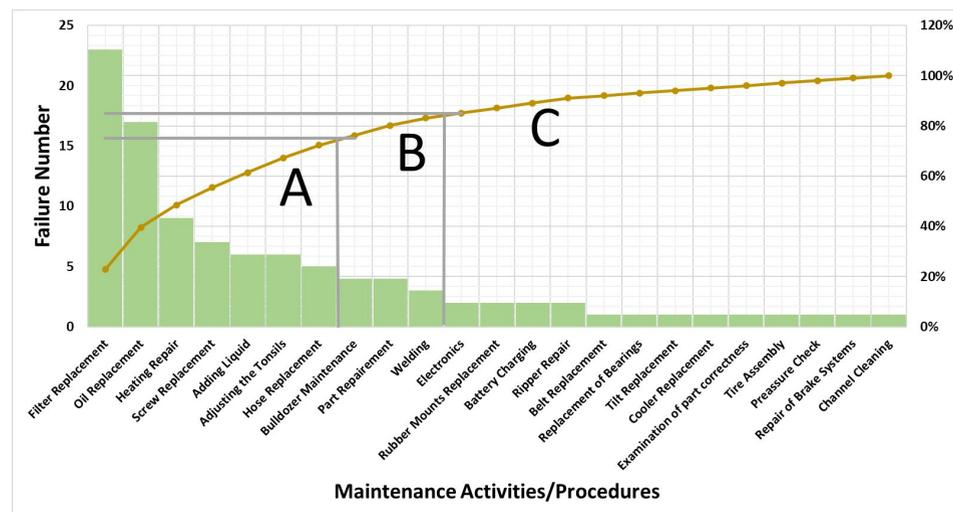
Figure 3: Pareto diagram of failures and stoppages for mining machinery.
