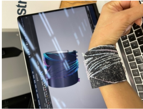
Figure 1: The image of worn bio-bracelet during wax removing, compare with the original 3D model.
