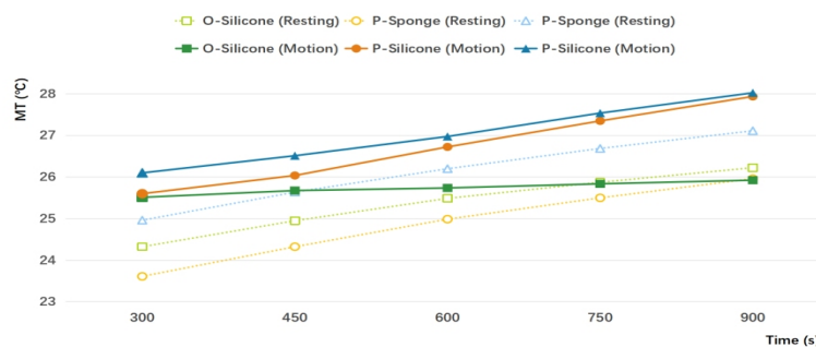
Figure 4: Average microclimate temperatures of three HMDs (°C).
