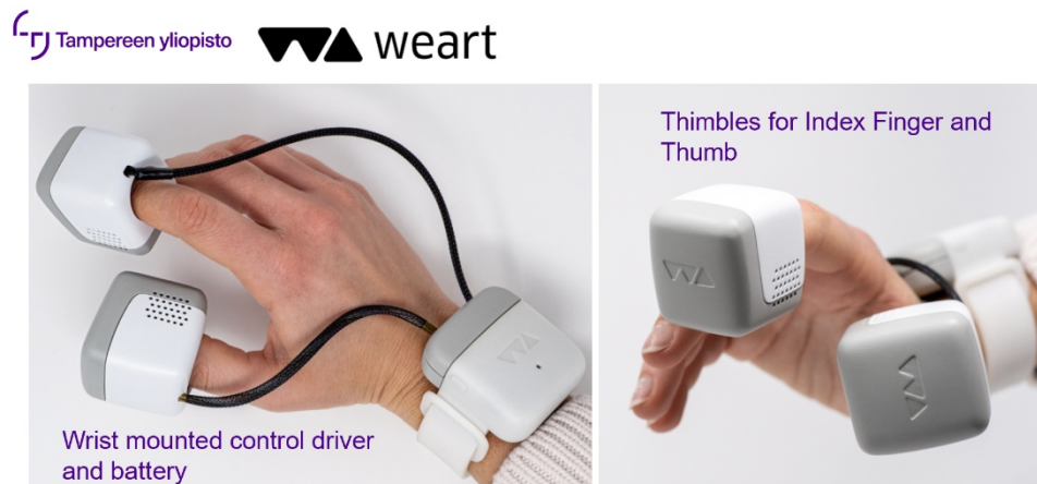
Figure 1: WEART Thimble device consisting of three wearable thimbles that can be worn on the fingertip (the distal phalanx that includes the perionychium, nail plate, and volar pad) along with the wrist mounted control trigger and battery bank.
