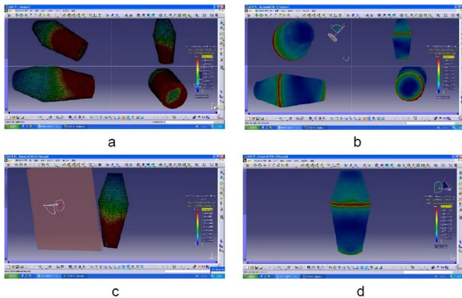
**Figure 5:** Visualization of nodal values of Von Mises stress for a. FM1, b. FM2 and sections c. FM1 and d. FM2 requested at 8bf. Request: direction – wide-shore.
