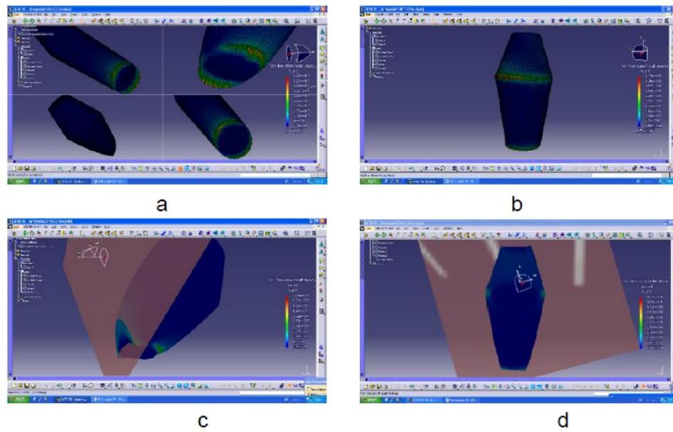
**Figure 4:** Visualization of nodal values of Von Mises stress for a. FM1, b. FM2 and sections c. FM1 and d. FM2 requested at 4bf. Request: direction – wide-shore.
