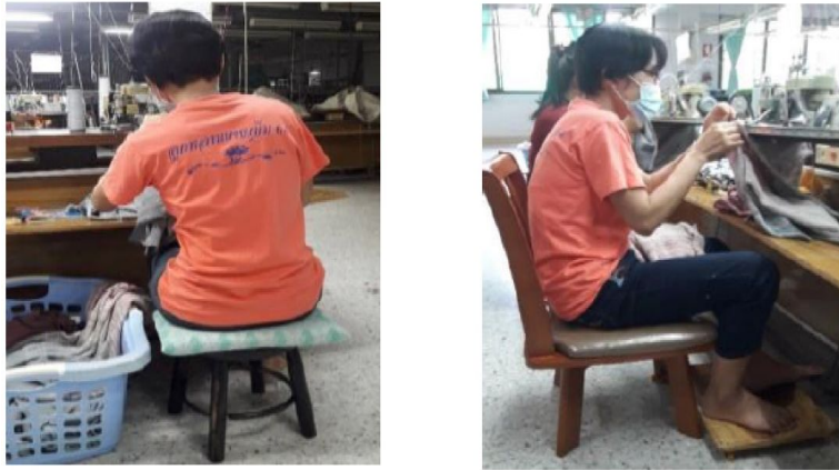
Figure 5: A worker sitting at a workstation in the sewing section before (left) and after (right) implementation.
