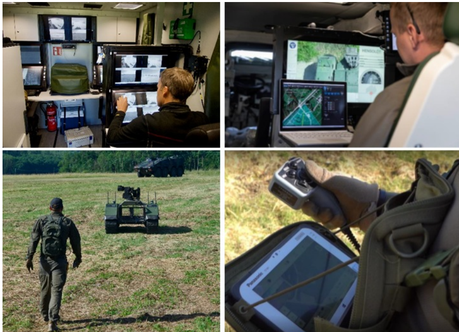
Figure 2: iMUGS human robot interfaces. Top: mission planning system in the boxer control vehicle. Bottom: one-hand control interface.
