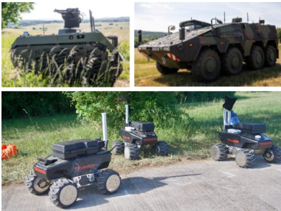
Figure 1: iMUGS robotic assets involved in the scenario. Top left: Milrem themis unmanned ground vehicle. Top right: boxer mission control vehicle; bottom: Robotnik Summit UGS swarm for resupply operations.
