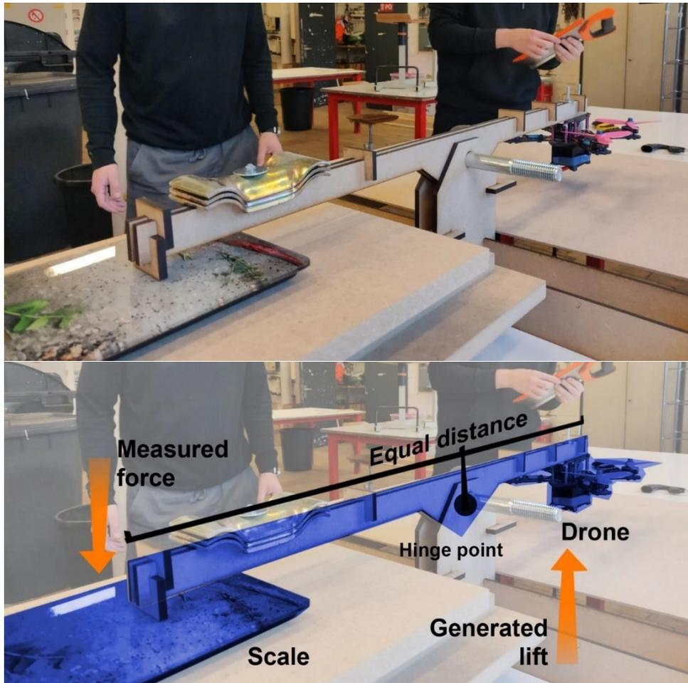
**Figure 2:** Picture of the set-up for the thrust-test.
