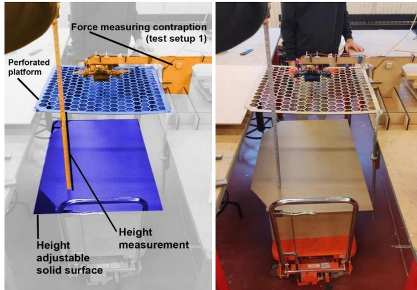
**Figure 3:** Picture of the set-up for the distance-test.
