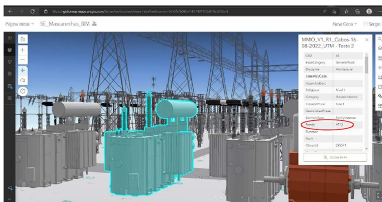
Figure 4: Navigation and access to the equipment attributes of the BIM model (Revit) of SE Mascarenhas in ArcGIS OnLine of Furnas.
