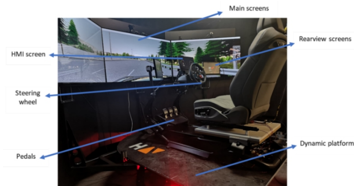
Figure 1: Driving simulator layout during the experimentation.
