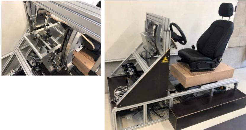
Figure 3: Steering wheel adjustment module and seating buck.
