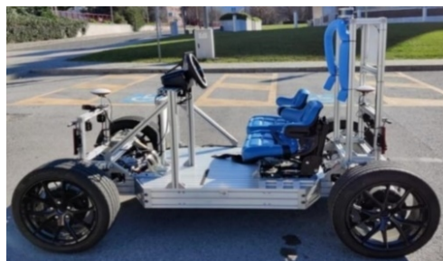
Figure 1: The autonomous vehicle with level 2 which was used in the experiment.
