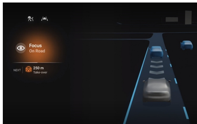
Figure 3: HMI of active ADAS functionality (condition 3a) that is triggered by driver distraction. a warning to focus on the road is issued, time gap to lead vehicle is increased and shown to driver by adding arrows between lead and ego vehicle.
