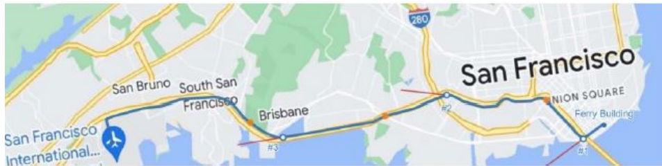
Figure 2: Sample route, highlighted in blue, to/from the SFO airport and the Ferry vertiports with the diversion points indicated by the white circle along the route. The orange circles represent the target point to re-engage the autopilot.
