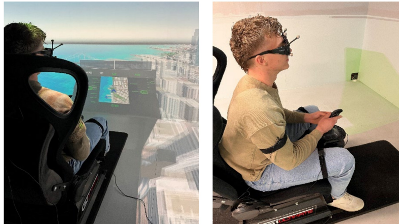
Figure 1: Right: side view of pilot seated in the CAVE simulator with tactors placed on the arms and thighs. Left: back view of pilot seated in simulator with cockpit display and out-the-window view.
