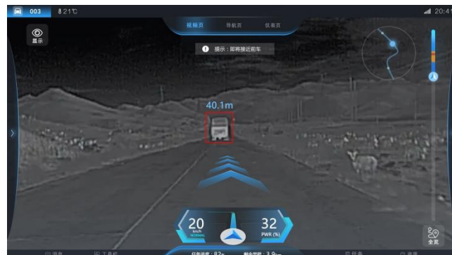
Figure 4: Distance early warning.
