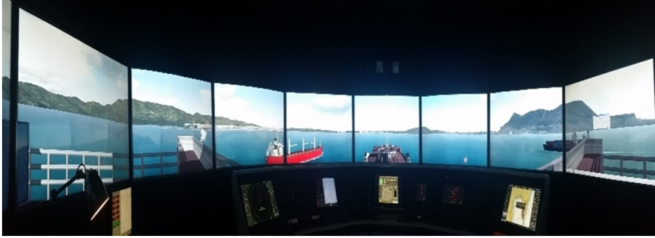
Figure 2: Navigation simulator (TRANSAS NT- PRO 5000).
