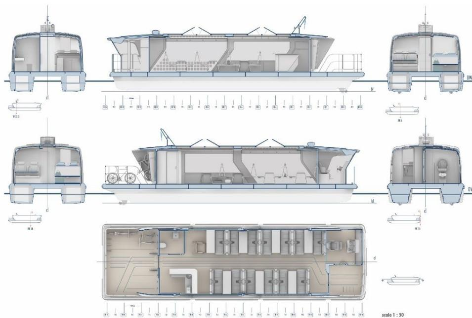
**Figure 5:** ZEUS 2 – deck plan, sections (Cipressi, 2022).
