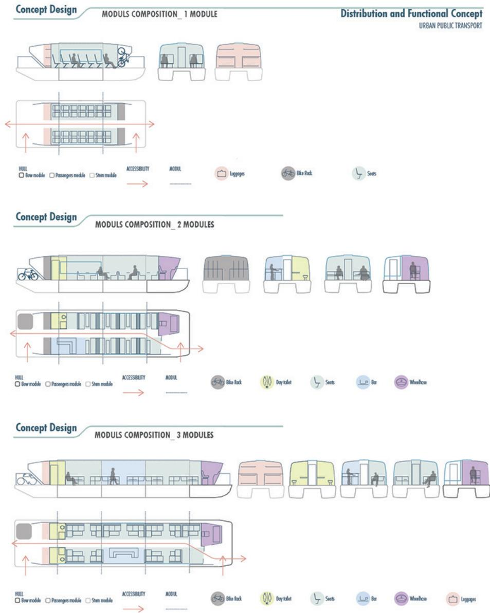
Figure 3: Modular design, platforms, and possible configurations (Cipressi, 2022).
