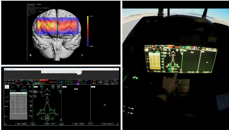
Figure 1: Screenshot from the LAD layout assignment task before the taxi phase. Video streams display the prefrontal oxygenation changes (top-left), the LAD screen feed (bottom-left), and the eye-tracking world camera view overlaid with a gaze indicator (right).
