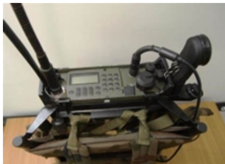
Figure 3: RRC-9200A radio station with antenna [13].
