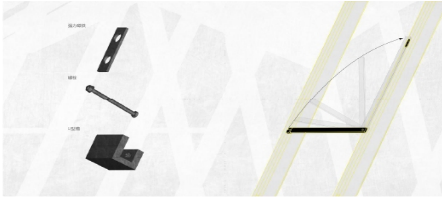
Figure 9: Hanging crossbar rotates through a combination of bolts and powerful magnets, allowing storage during weekdays when events are not held. (Self-drawn by the author).
