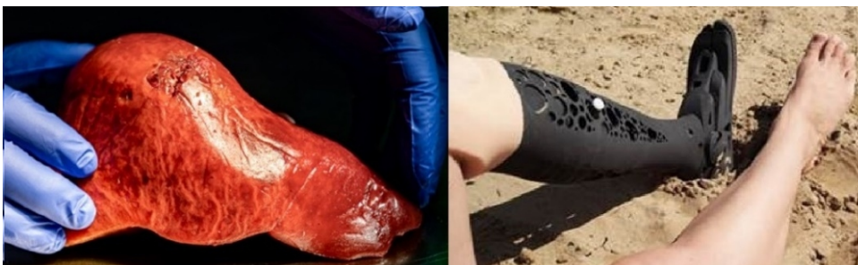
Figure 1: Left: realistic liver phantom (hybrid: 3D-printing/collagen cast) with sensor integration (cirp GmbH for VIVATOP project). Right: SLS 3D-printed prosthesis (cirp GmbH, ©Fraunhofer IPA).
